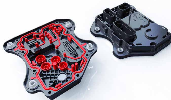
Multi-component housing made of thermoplastic with molded-on seal made of liquid silicone rubber for an electronic control unit in vehicles.
