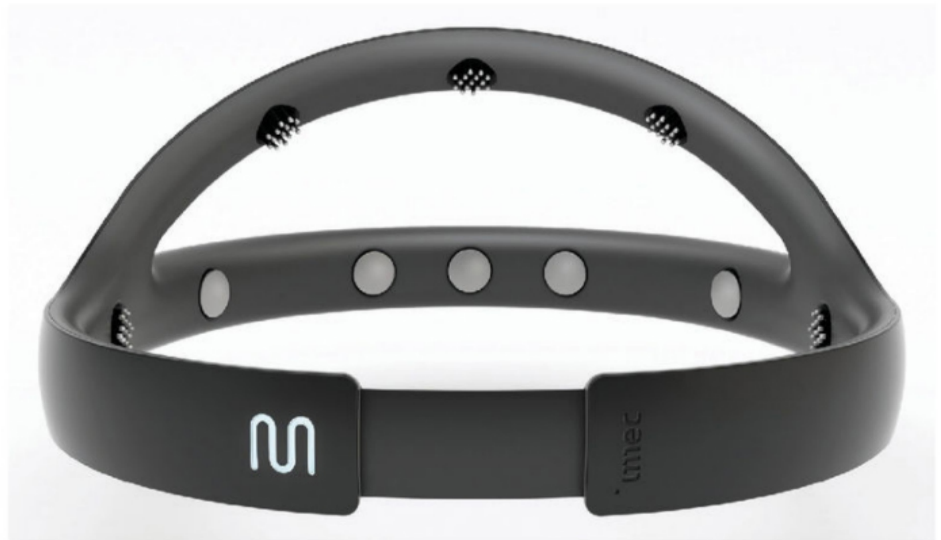
Imec's prototype of a wireless EEG headset, measuring EEG signals with clinical quality.
